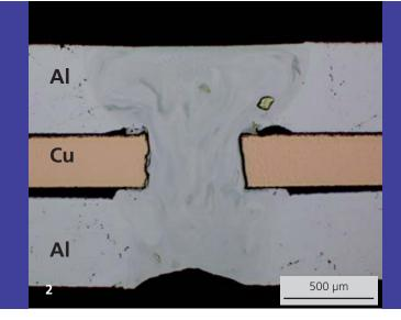
With this technology, a brilliant laser beam is deflected over quickly tiltable mirrors and projected on to the joining impact. The good focusability of high-brilliance laser beams makes it possible to obtain extremely narrow welding joints with high aspect ratios and extremely short melt pool operating cycles. The energy input into the work-piece is thereby considerably reduced and the formation of the brittle intermetallic phases significantly decreased.
